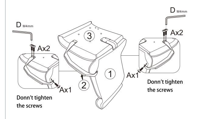
STEP 5: Connect mechanism 4 to seat 3, use hexagon socket wrench D to twist screw B, and finally tighten all screws.
