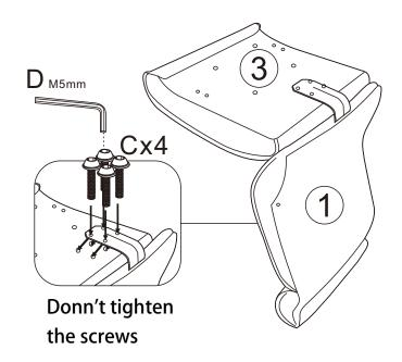
STEP 4: Connect armrest 2 to seat 3 and back 1, and twist into screw A with inner hexagon wrench D.
